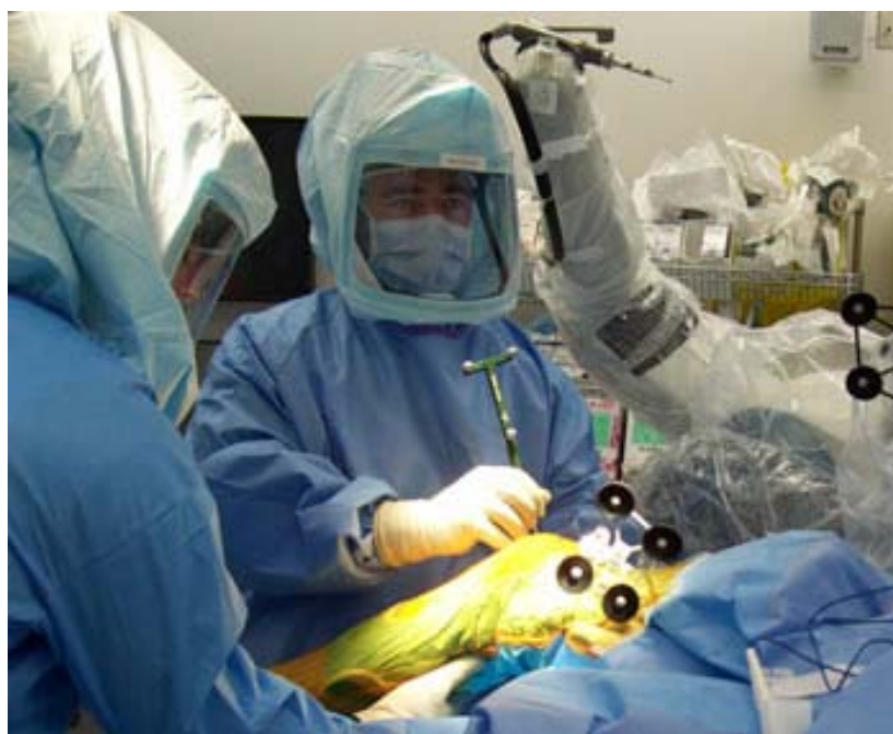
Figure 2-14: Bone registration is performed by using a tracking probe to collect data points directly on the bone surface (Copyright. Picture retrieved June 19, 2011, from http://www.texashealth.org/body.cfm?id=4169 ).
