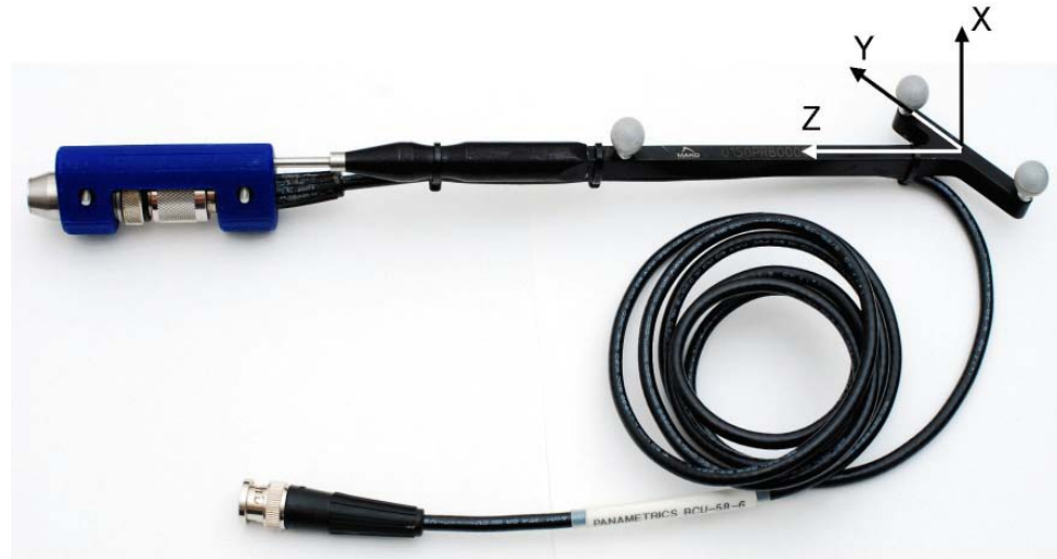
Figure 3-5: A-mode US probe was made by attaching the US transducer to the tip of a mechanical probe along the long axis.
